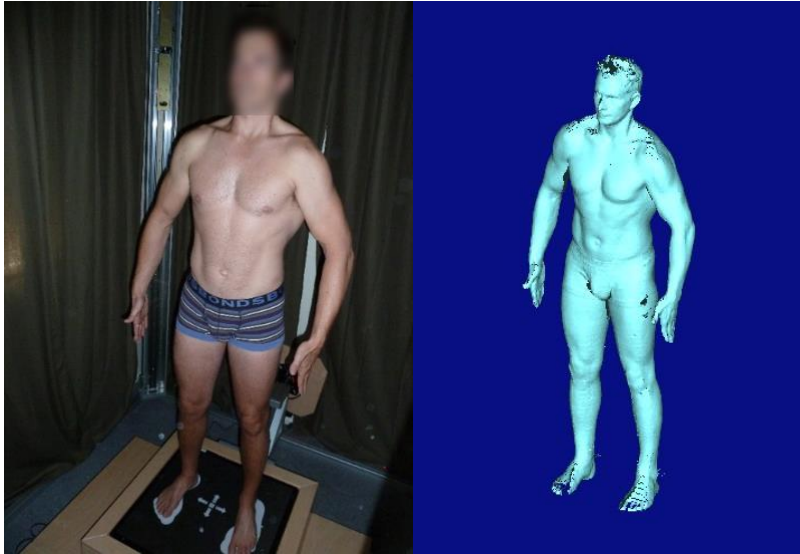
Figure 9. An example of a scan posture within the Vitus XXL. Body postures vary from participant to participant and if not controlled, is a potential source of measurement error.
