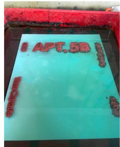
Figure 13. Etching Metal.
