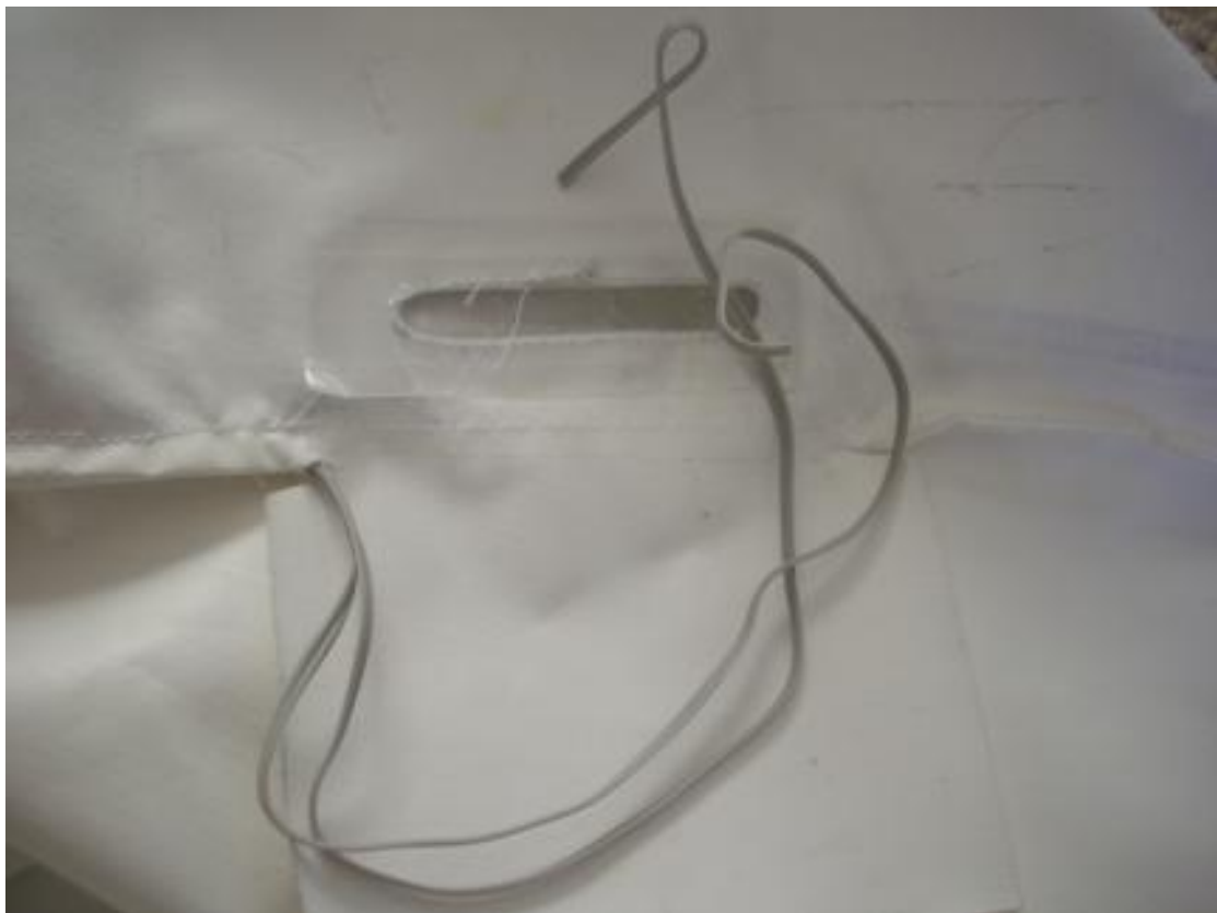
Figure 18. Inside detail showing French seam and cables
