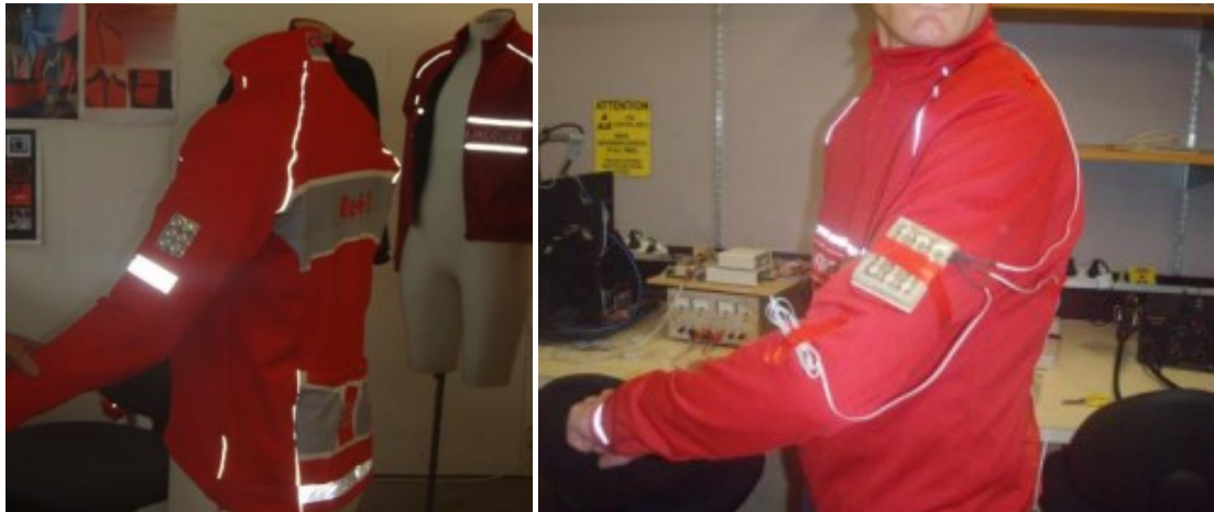
Figure 5. Cable and circuit board placement
