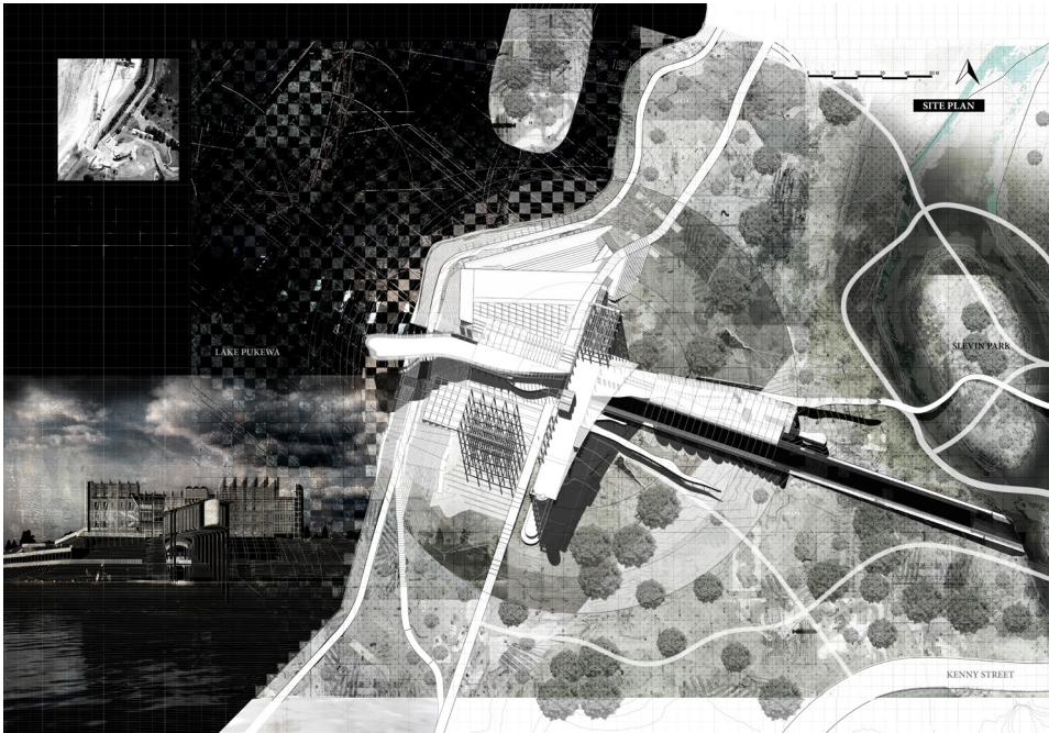
Fig. 11 Author (2021). The Vessel: Site plan. The water enters the lake through the newly formed passage which flows beneath the building. [Digital drawing]
