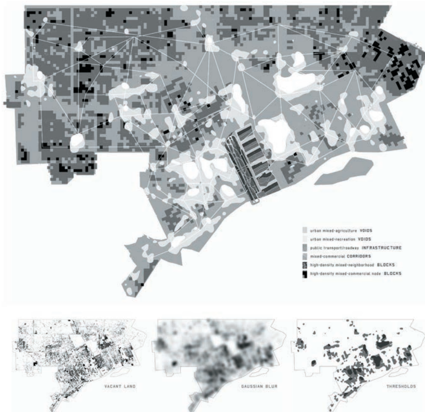
Figure 2: Detroit City-State plan. Areas of urban void, urban densification, in-between, new infrastructure, and proposed downtown airport location. Bottom left: existing land vacancy. Bottom middle: Gaussian blur filter applied. Bottom right: Threshold filter applied, determining extent of urban agricultural and urban recreational voids.
