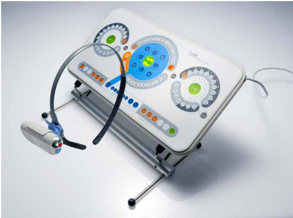
FIGURE 2. LOMAK (Light Operated Mouse and Keyboard). Designed by Peter Haythornthwaite and held in the New York Museum of Modern Art's permanent collection.
