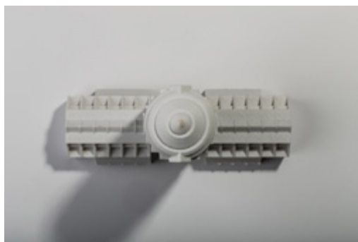
Figures 19-20: Scale model of Lambton Tower interpreted from National Library collection material and 3D printed in white ABS
